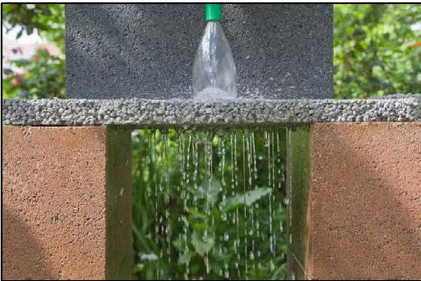
*Image (left) shows the high porosity of pervious paving, which allows water to filter slowly back into the ground, reducing the amount of runoff and drainage into the sewer system.*
